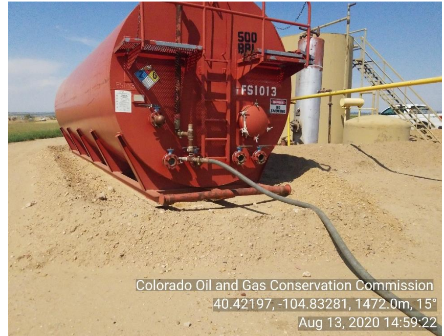
Photo 10: Tank not grounded
