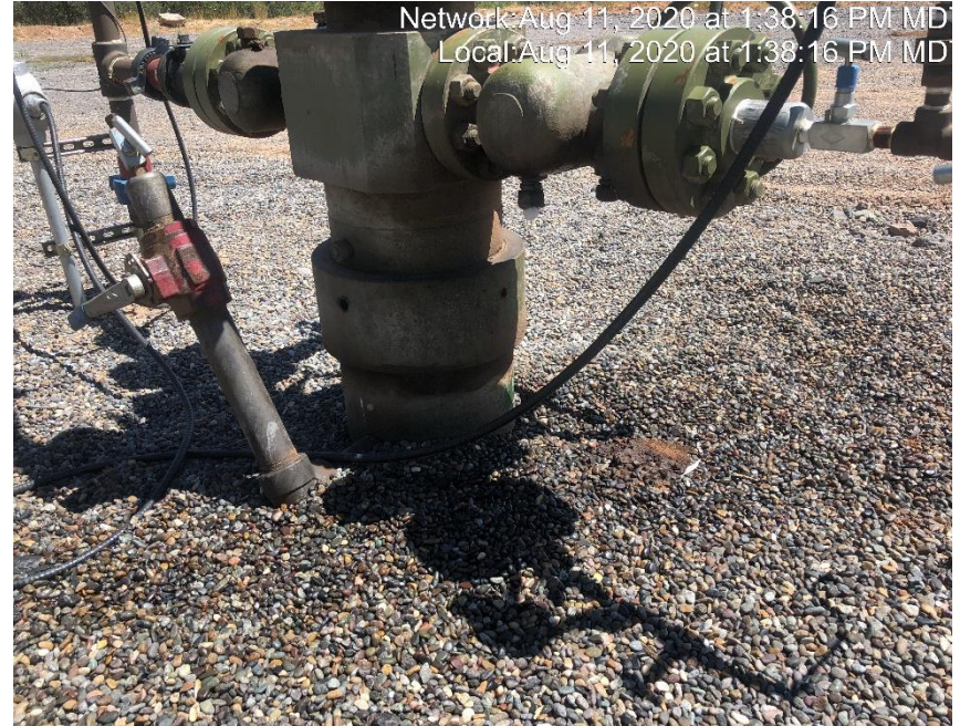
Photo #1705 Stained soil at wellhead.
