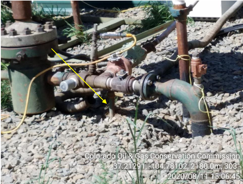
PHOTO 5: UNUSED 1" RISERS NEXT TO WELLHEAD UNDER 2" PRODUCTION LINE. REMOVE UNUSED RISERS, COMPLY WITH RULE 603.f. CA DATE 11-11-20.
