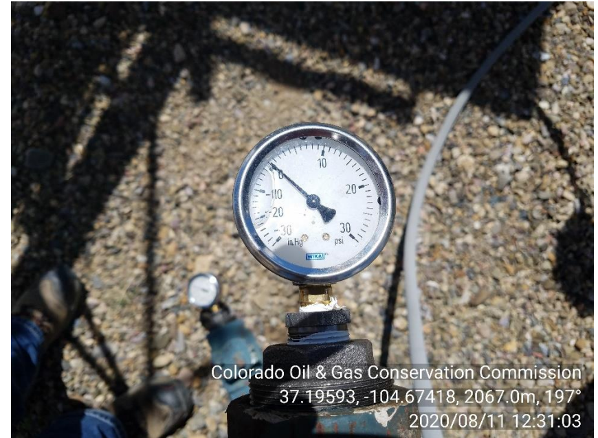
PHOTO 4: ANNULUS BETWEEN TUBING AND CASING GUAGE.
