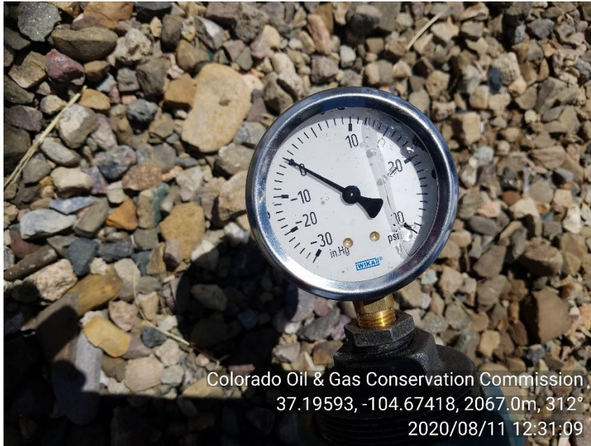
PHOTO 5: BRADENHEAD PRESSURE GAUGE
