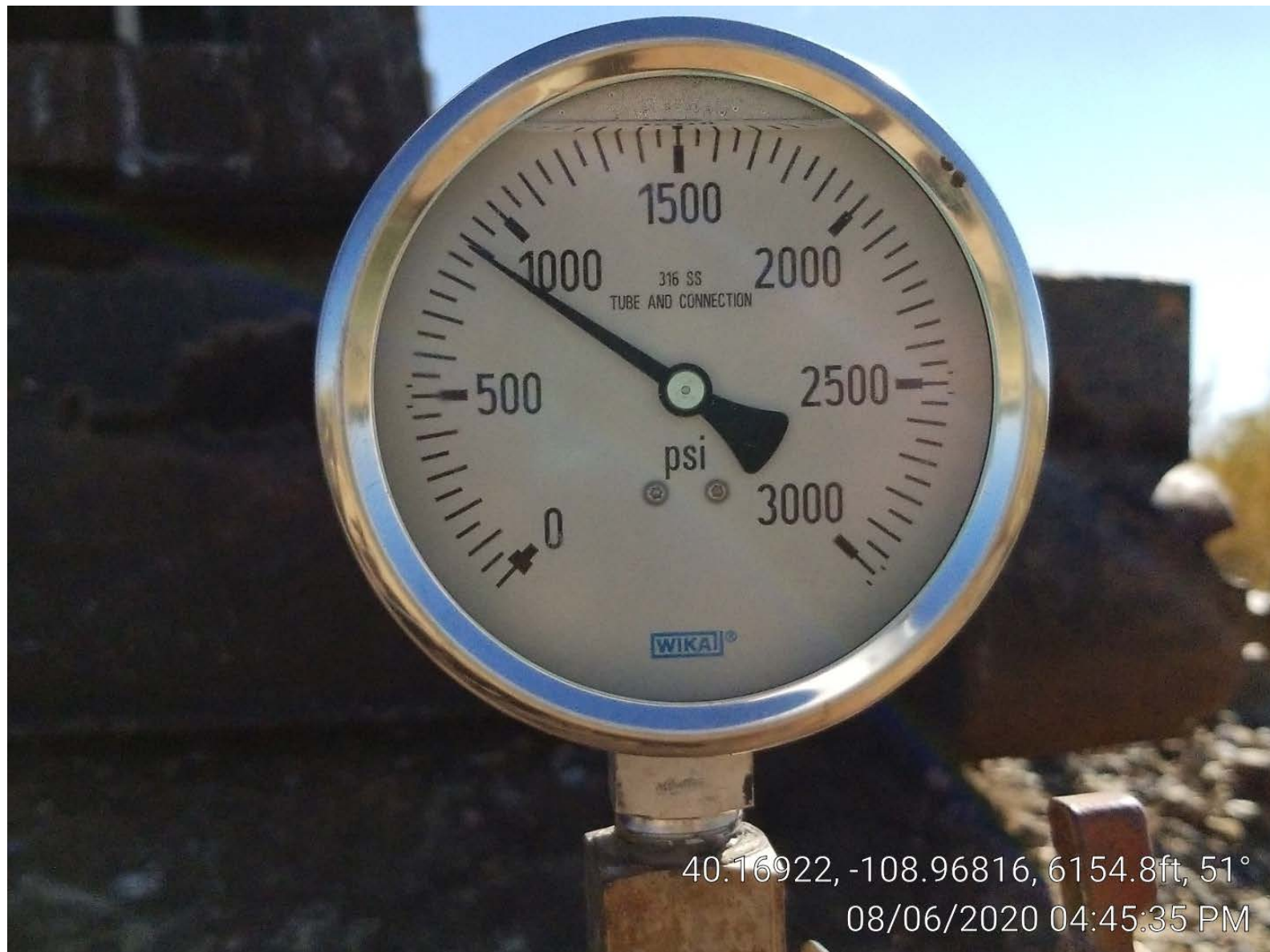
Photo 9. Casing gage.
