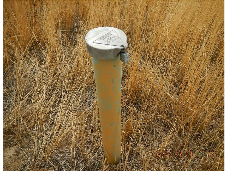
MW located in the NE corner of the facility. This is the only MW that was secured with a lock.
