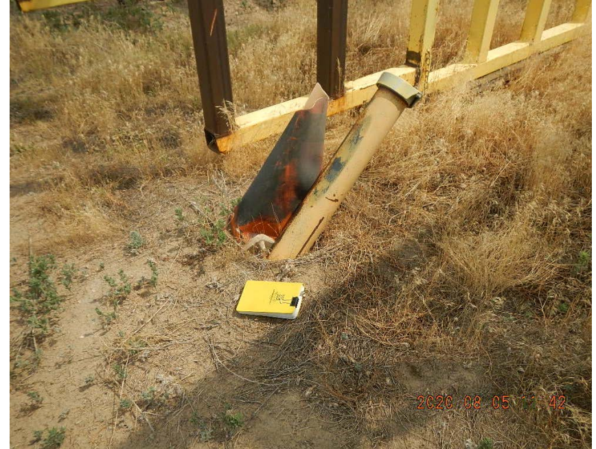
Damaged monitoring well.
