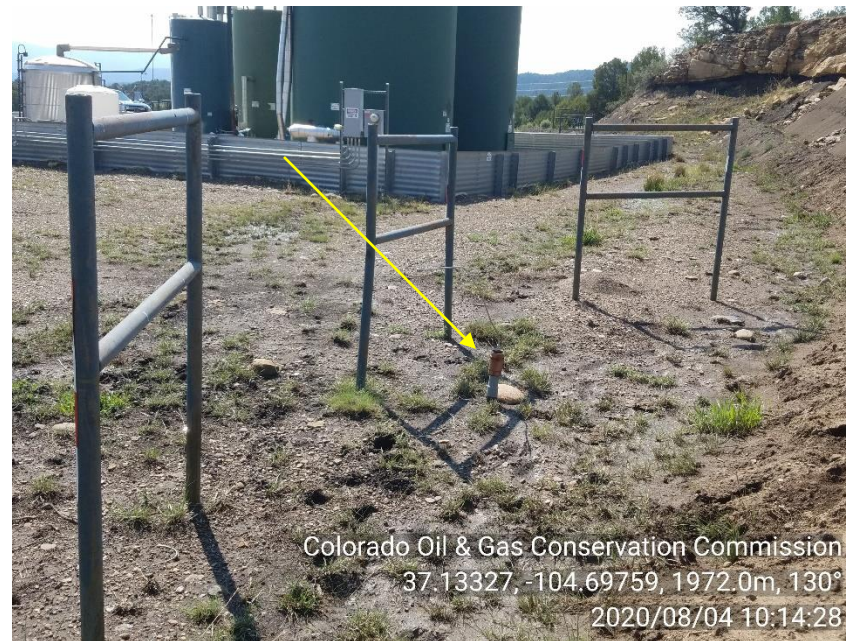
PHOTO 4: UNUSED EQUIPMENT (2" RISER NORTH WEST OF TANK BATTERY). REMOVE RISER OR PUT INTO USE. CA DATE 11-4-20.
