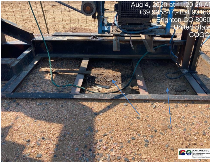
Pic 5 stained soil under pump jack motor
