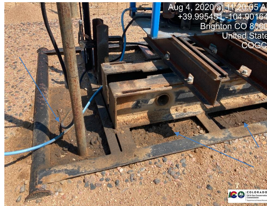
Pic 4 Stained soil around pump jack motor
