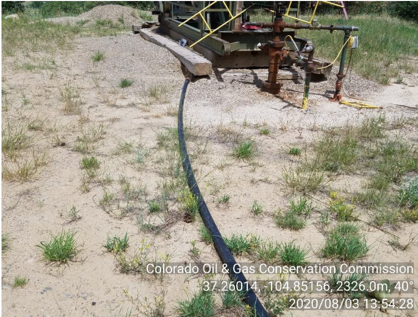
PHOTO 3: UNUSED EQUIPMENT STORED ON LOCATION (2" POLY PIPE). REMOVE UNUSED EQUIPMENT, COMPLY WITH RULE 603.f. CA DATE 11-3-20.
