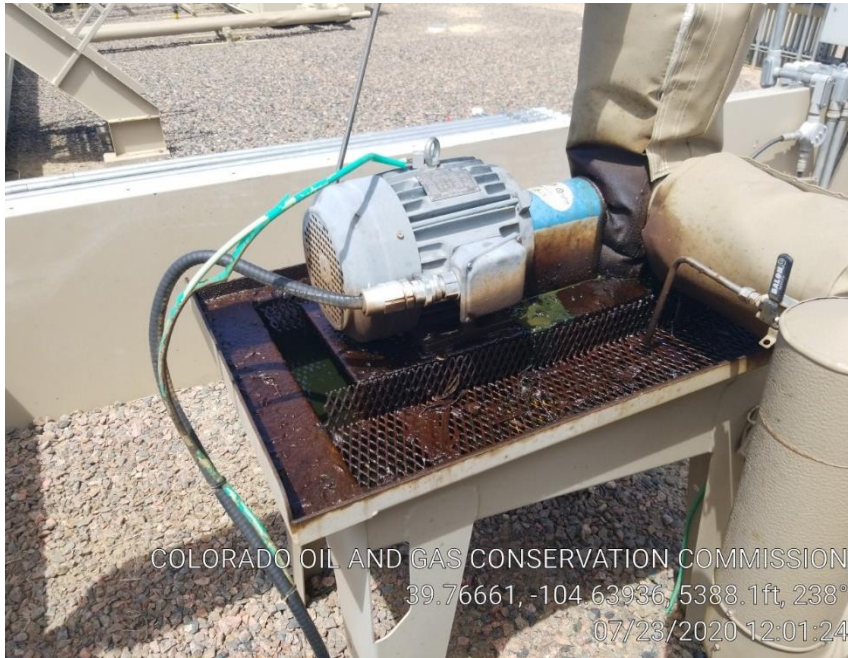
Pic 3 inadequate netting.
