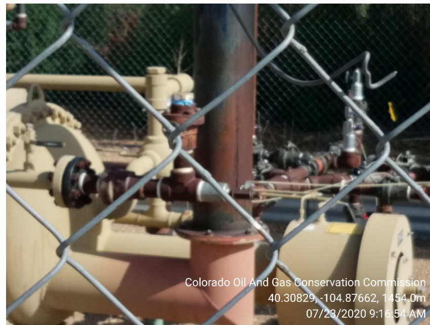
Disconnected separator gas sales line
