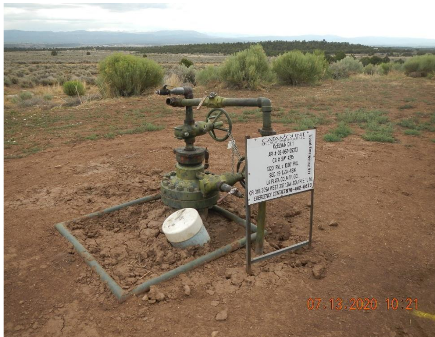
McElvain Dakota #1 well head. Flow line disconnected at well head.
