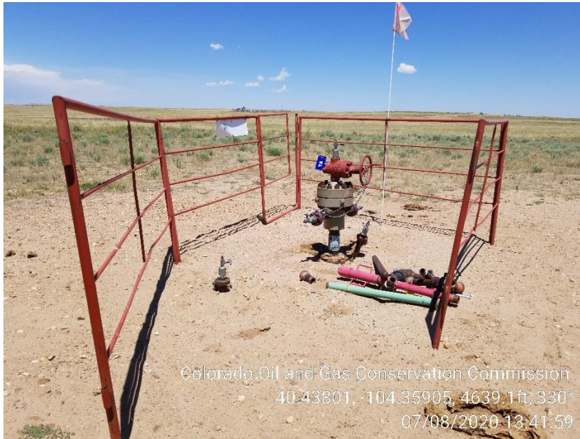
Photo 1 – Wellhead, unused WH parts
