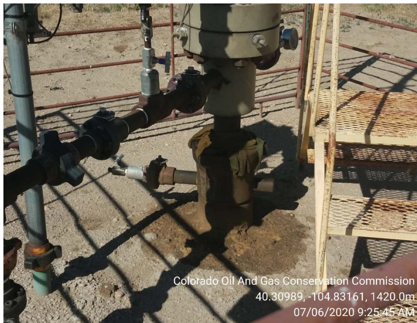
Bradenhead packing and stained soil
