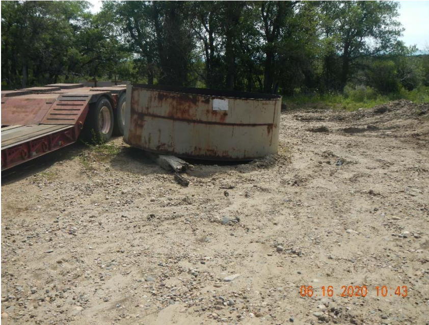
Photo 3. Tank stored without containment or labels.
