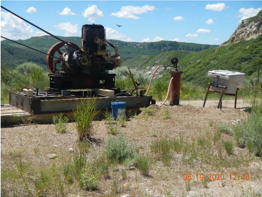
Photo 5. Lube oil stored without containment.
