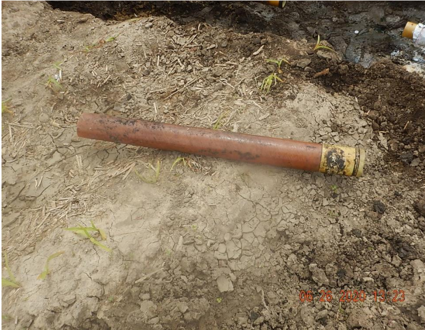
View of failed section of fiberglass pipe and fitting installed as part of repair completed by KPK in response to reportable spill ID #470915 submitted to COGCC on 1/17/2020.
