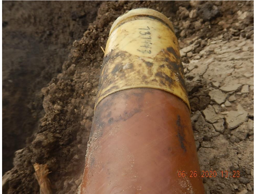
Closer view of fitting on cut end of pipe section; KPK crew informed COGCC Inspector a leak is suspected to have developed between fitting and outside wall of FG pipe. Integrity/ adhesion failure of the prior repair is suspected to have caused second reportable spill (#476987)
