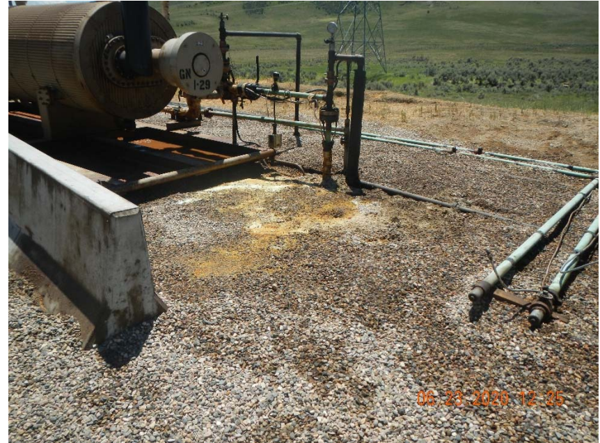
Photo 6. Stained soil from apparent spill.
