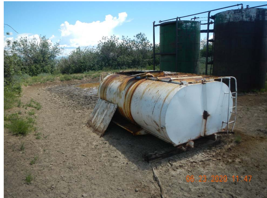
Photo 8. No label on tank. Stained soil at base.
