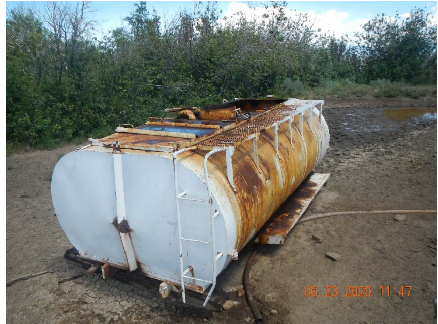
Photo 10. No label on tank. Stained soil at base.
