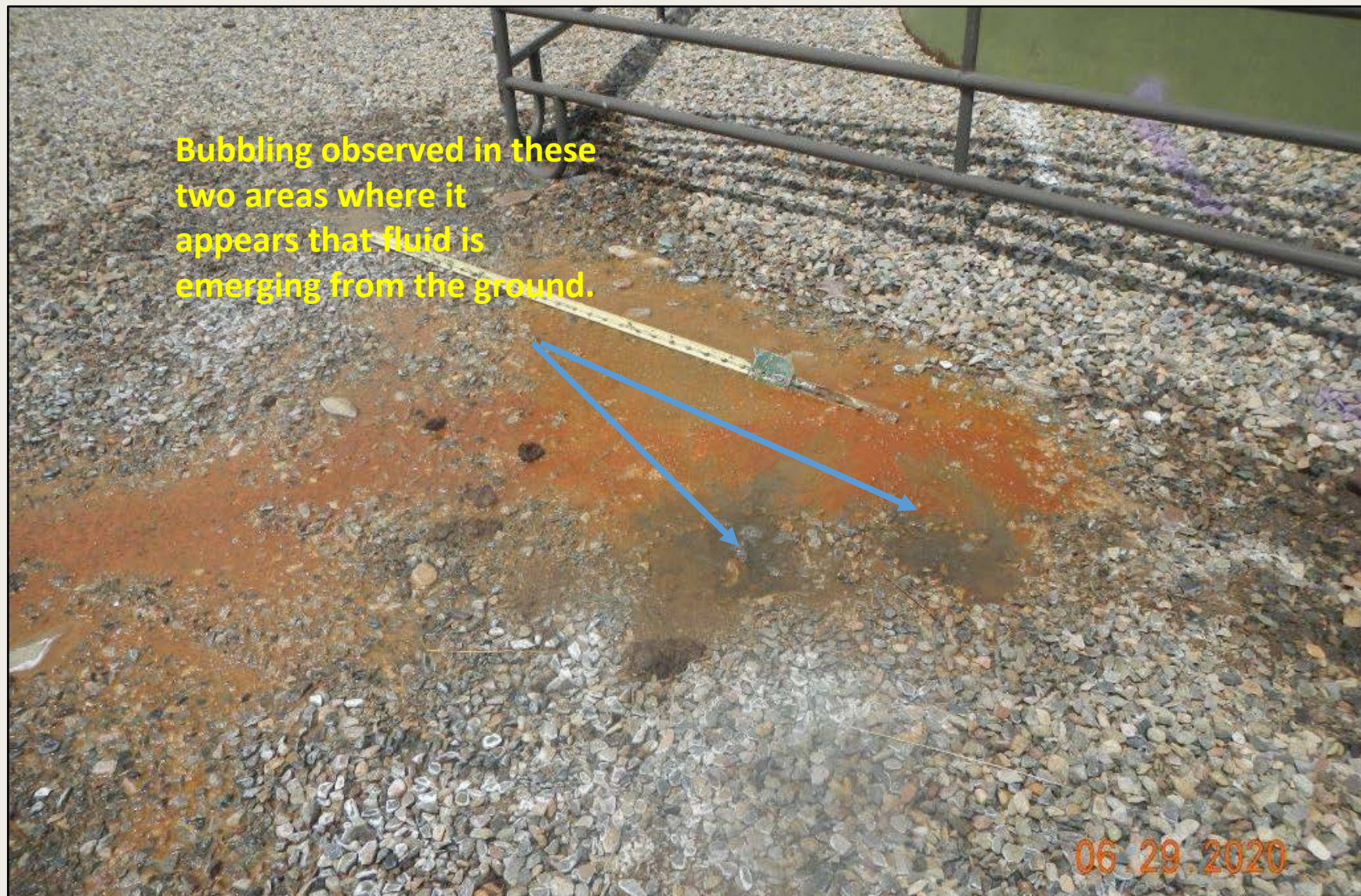
Photo 3. View of location where active release is emerging from the ground.
