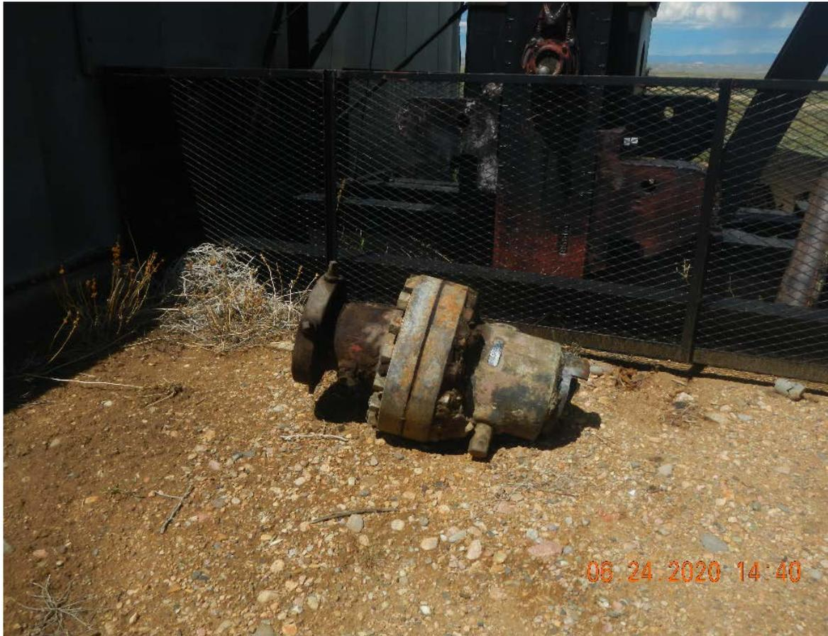
Photo #2 wellhead cut. Document review shows the well was indented to be PA on 8/12/2019
