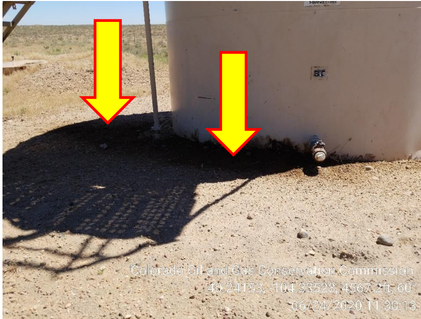
Photo 5 – Stained Soil at Crude Oil Tank
