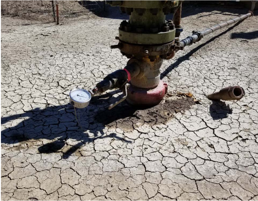
Photo #11 – Localized accumulation of oil-stained soil beneath wellhead. Note presence of mud cracks in wellhead area is indicative of stormwater pooling in this location.
