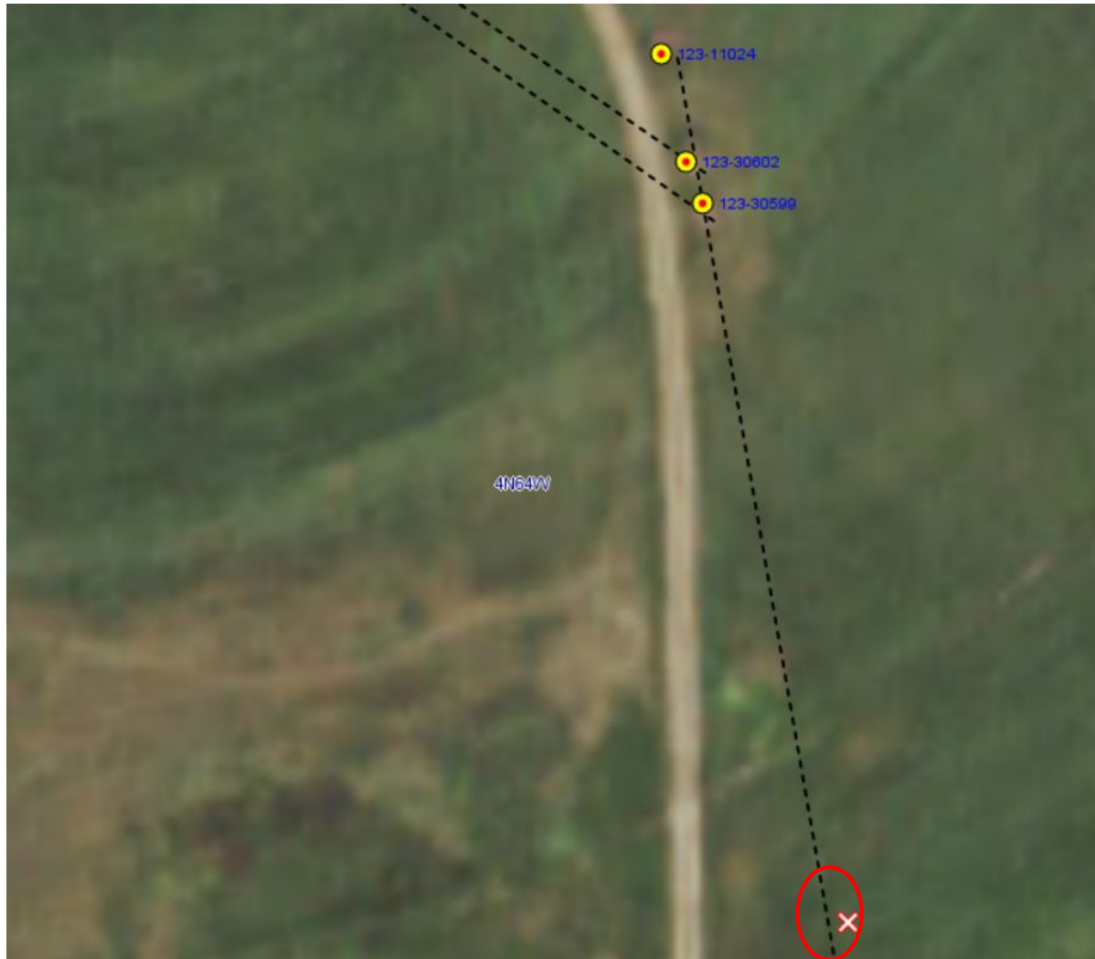
Photo 2. Aerial imagery taken in 2017. Aerial imagery of a subsidence area (red x) that appears to be associated with the flowline (black-dashed line= Active (inferred)) for well 123-11024. Subsidence is located at the approximate Lat/Long coordinates: 40.321403, -104.539956.
