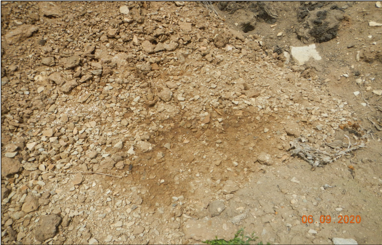
Photo 9. There is oil stained soils in the soil pile at the northeast side of the location. The soil had an oil odor.
