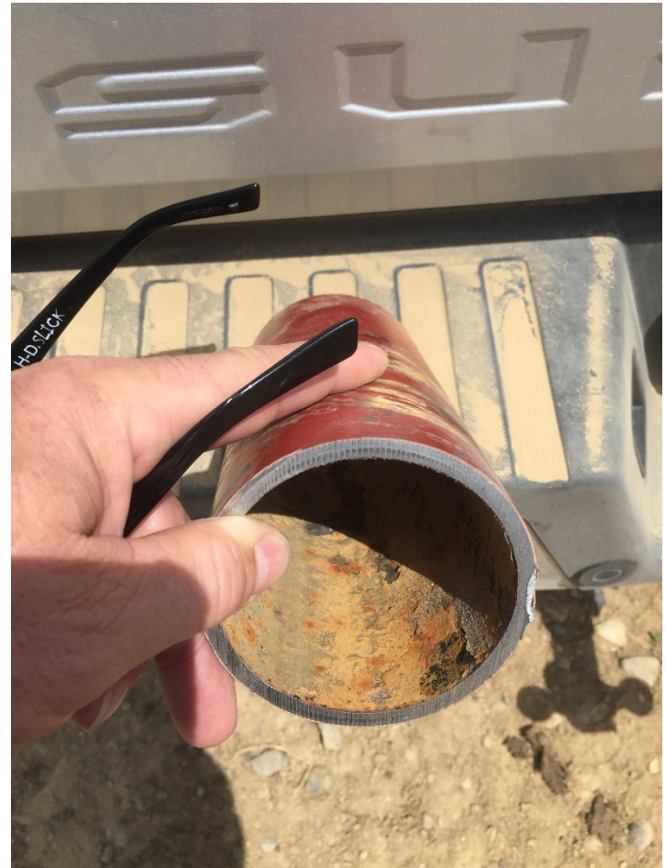
Pinhole found in flowline in the 3 o'clock position
