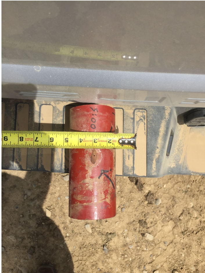
Pinhole found in flowline in the 3 o'clock position
