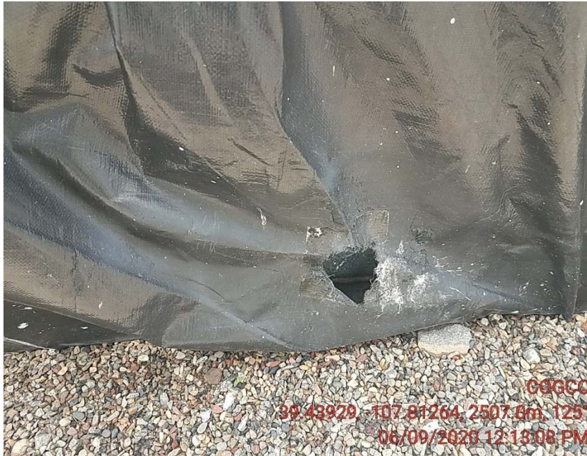
Holes in containment
