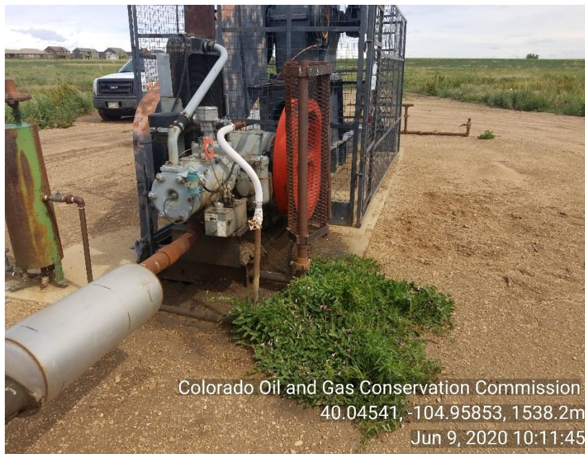
Photo 2 Stained soil under and around PU motor
