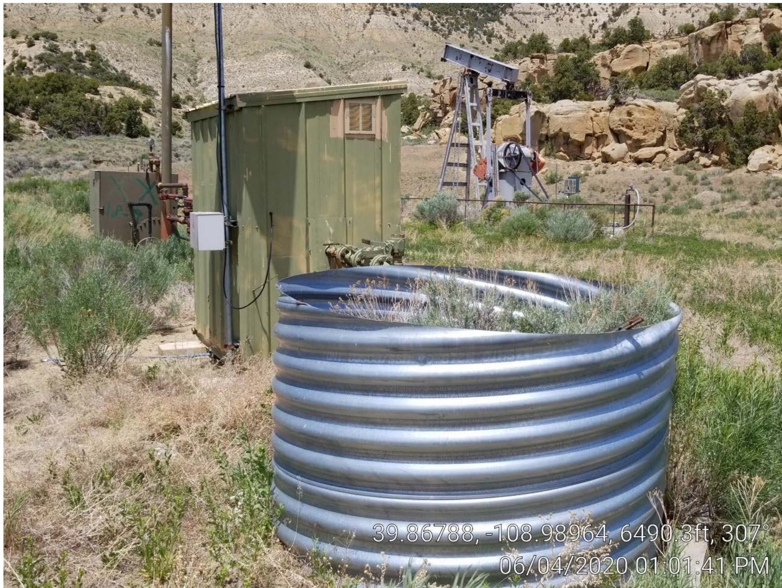
Photo 5. Culvert, meter building, separator, and pump jack.
