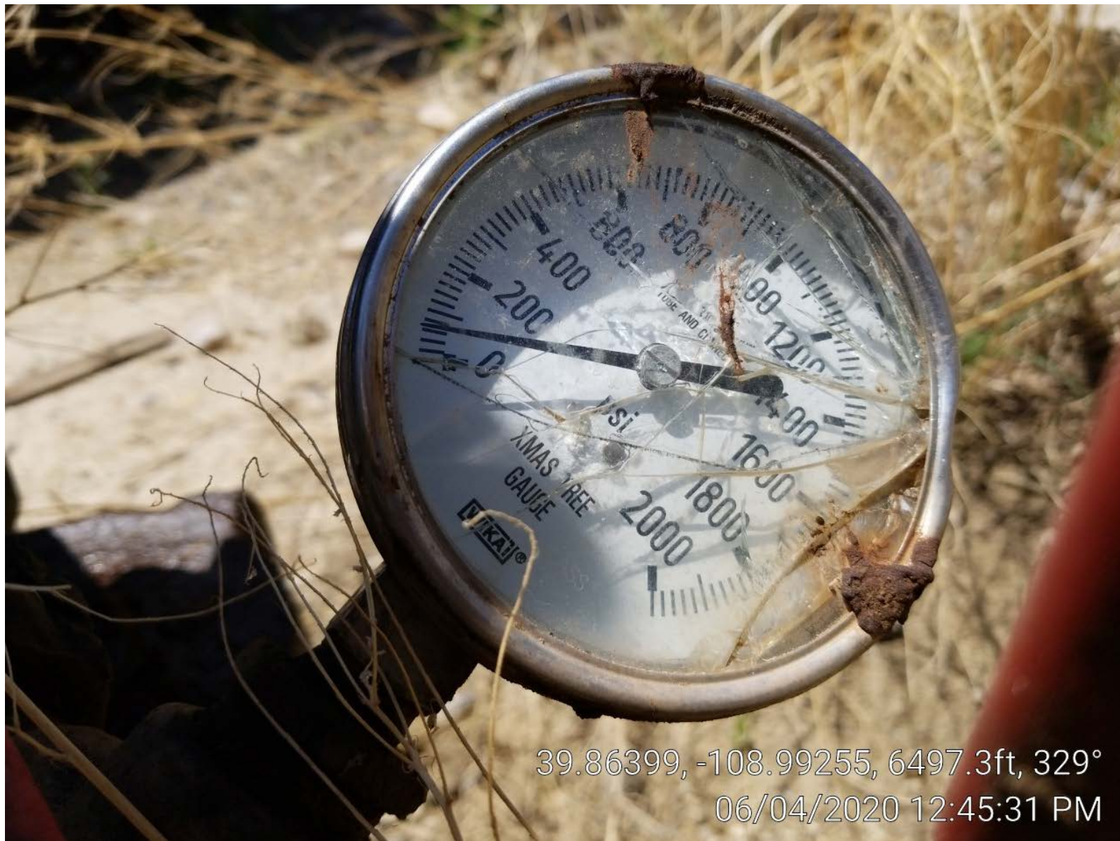
Photo 16. Tubing gage at 40 psi.
