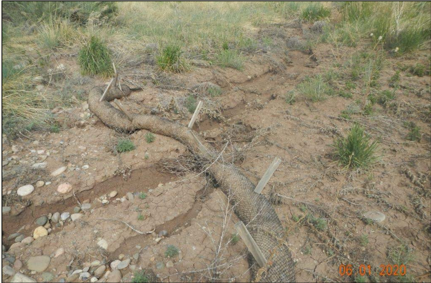
Photo 3. View of erosional channeling in Photo 2, facing downstream. Erosional channel is approximately 2 feet wide and 1 foot deep.
