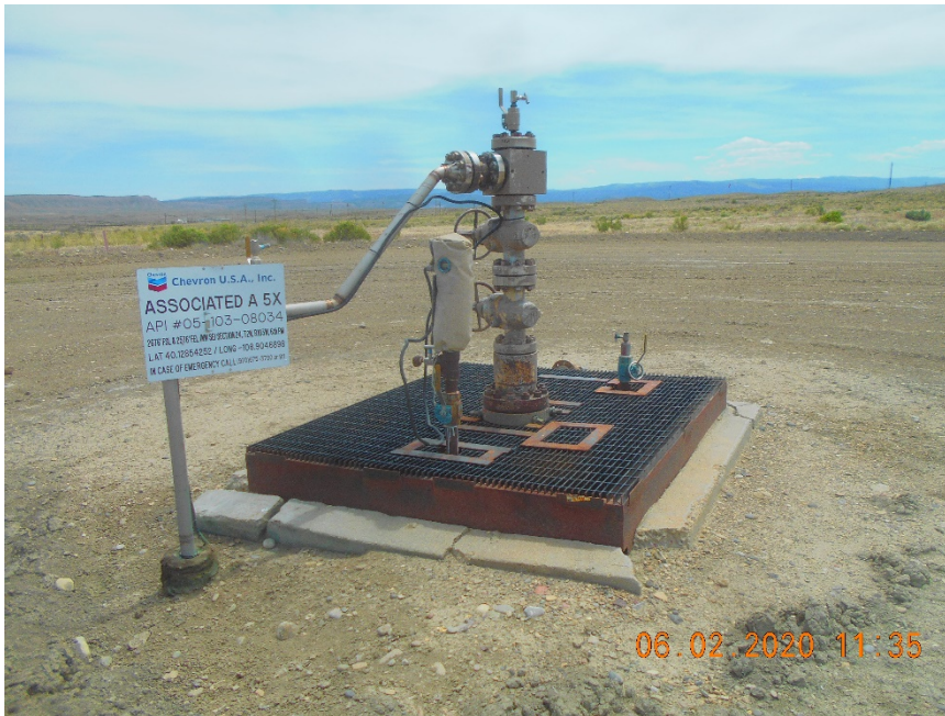
Injection wellhead.
