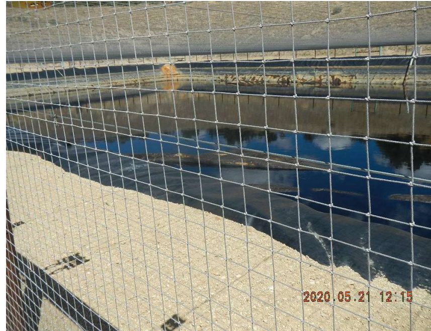
Free board at 10-12 feet from top of pit, and fluid surface 100% covered with hydrocarbons.
