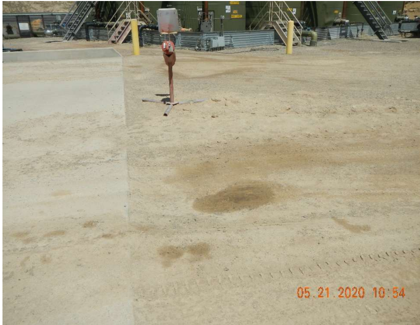
Localized accumulation of oily waste
