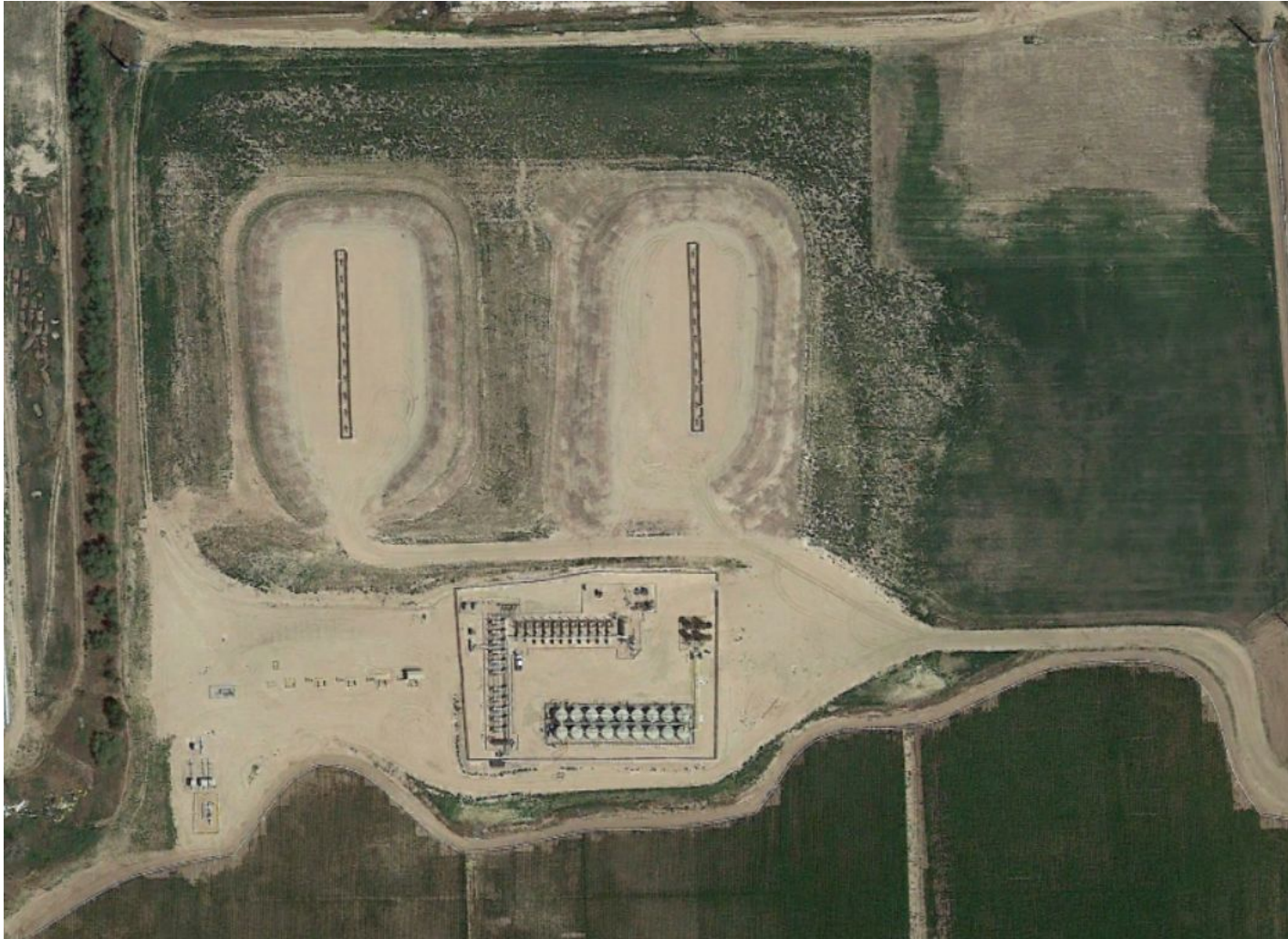
Photo 2. Google Earth aerial imagery taken 7/17/2019 after all 22 wells have been on production. Imagery illustrates Operator has performed interim reclamation activities to reduce disturbance areas only needed for production operations.
