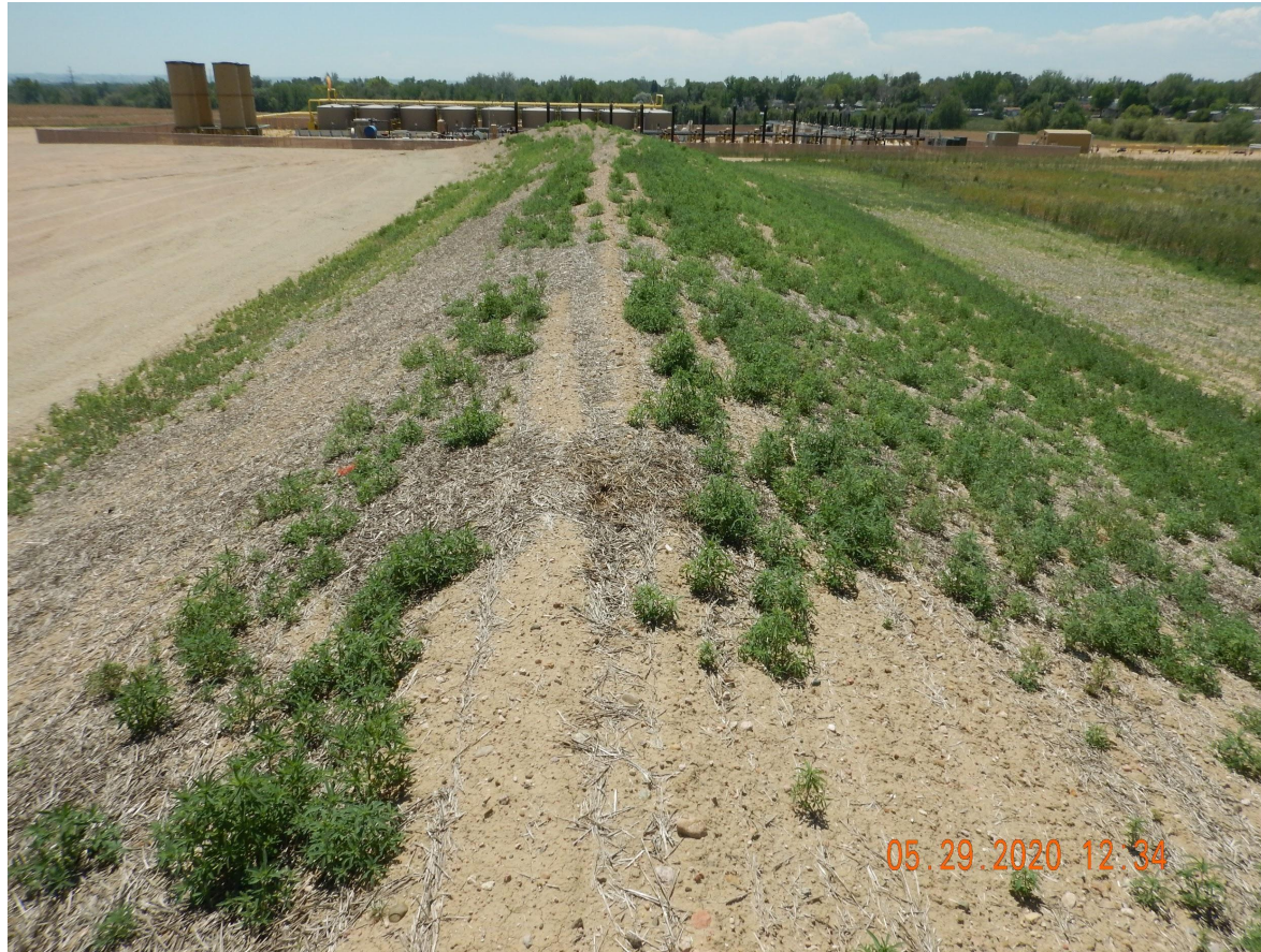
Photo 4. Photo taken from the eastern set of wells, facing South. Photo illustrates a stockpile that has been temporarily stabilized with equipment tracking. Operator has attempted to seed into the stockpile with the evidence of drill rows and straw crimped mulch. However, there was little establishment of desirable species and currently has mostly Kochia establishment.
