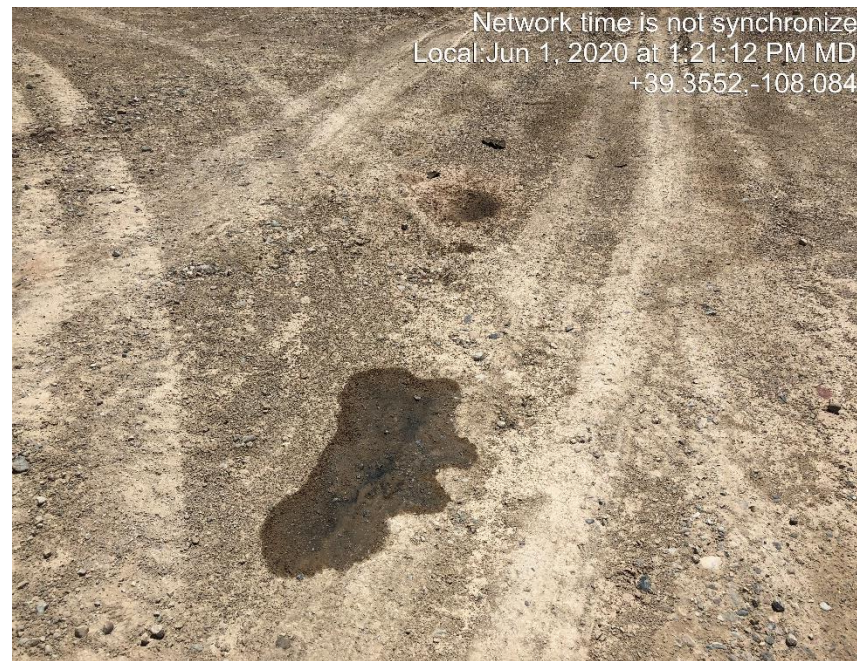
Photo #1288 Stained soil outside of tank containment.
