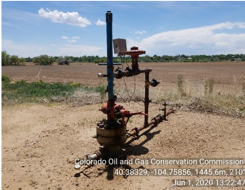
Photo 1: Wellhead, NO SIGNAGE
