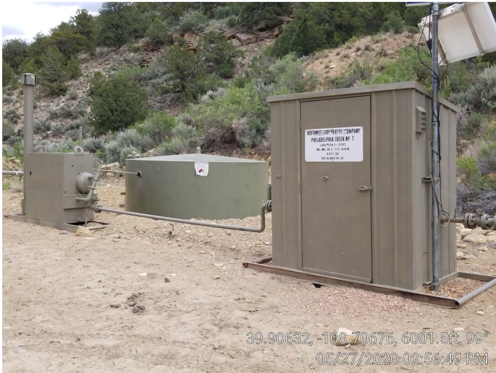
Photo 3. Separator, tank, and meter building.
