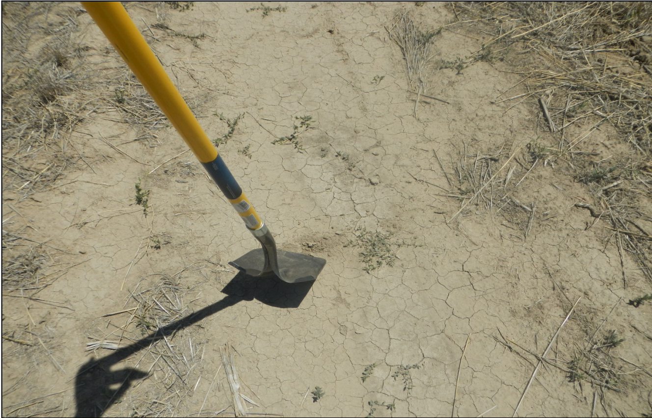
Photo 3. The shovel was used to test for soil compaction along the access road and location. The soils were compacted and the shovel was not able to penetrate the surface with pressure.
