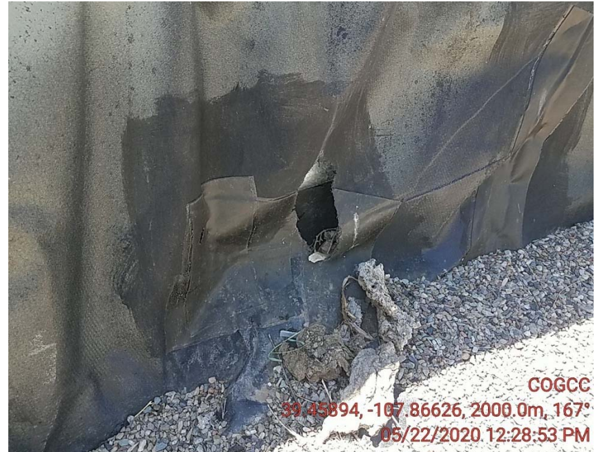
Holes in containment
