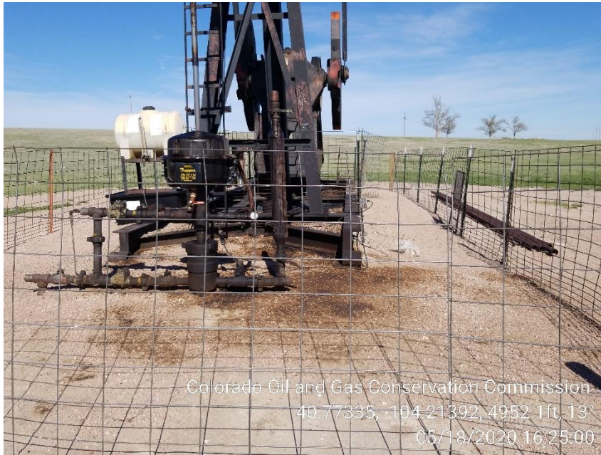
Photo 3 – Stained Soil at Wellhead
