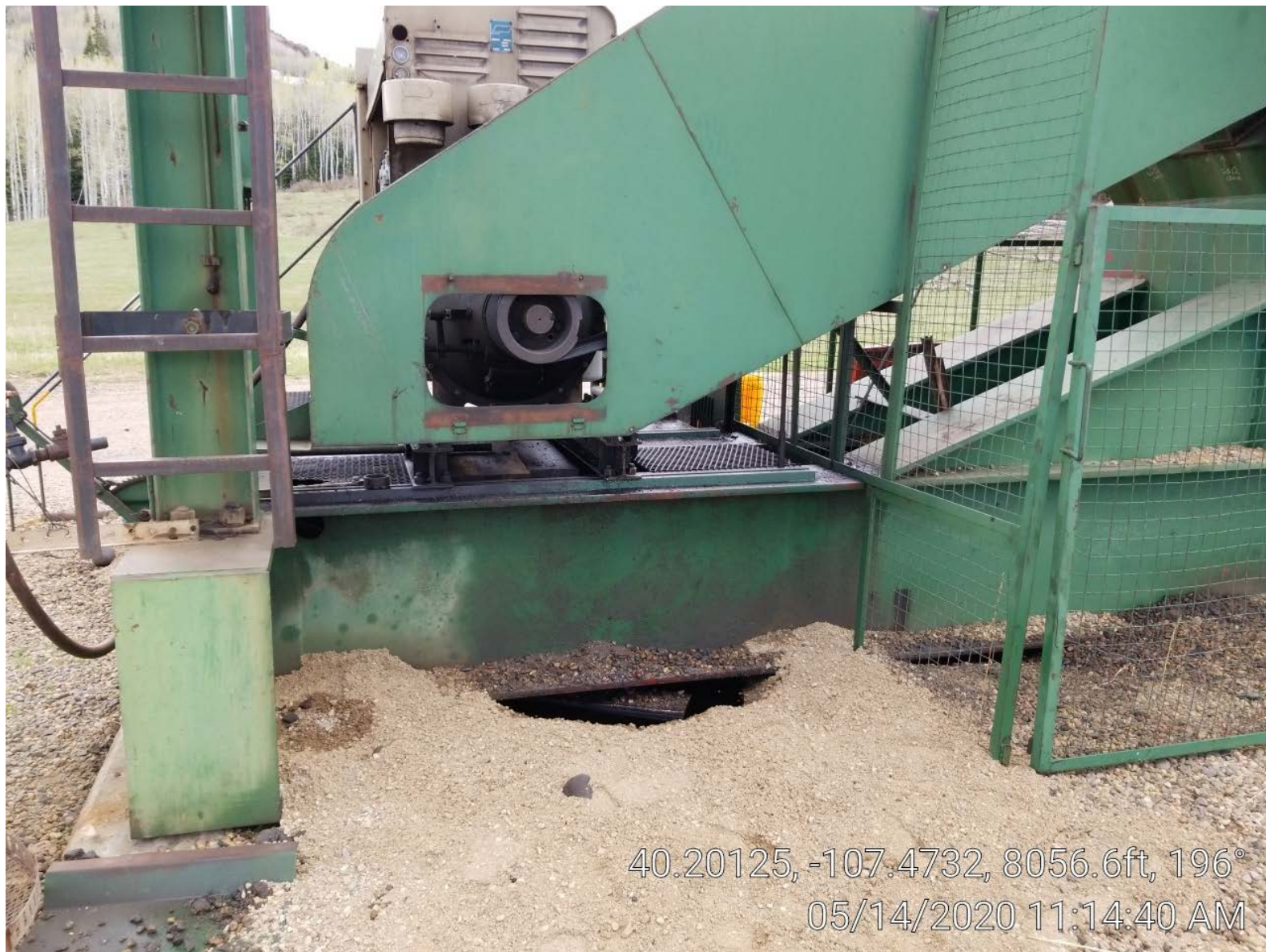
Photo 11. Side of pump jack. Oil on ground partially covered by recent dirt.
