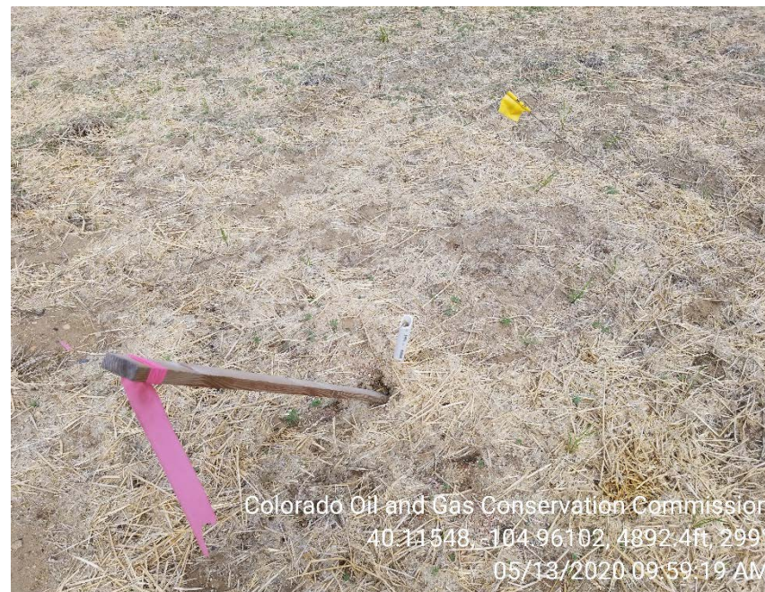
Photo 2 – Monitoring well; damaged and uncapped
