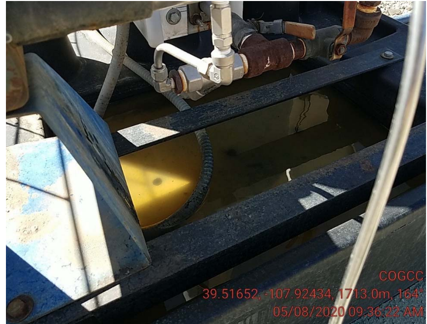
Chemical containment is full of liquid
