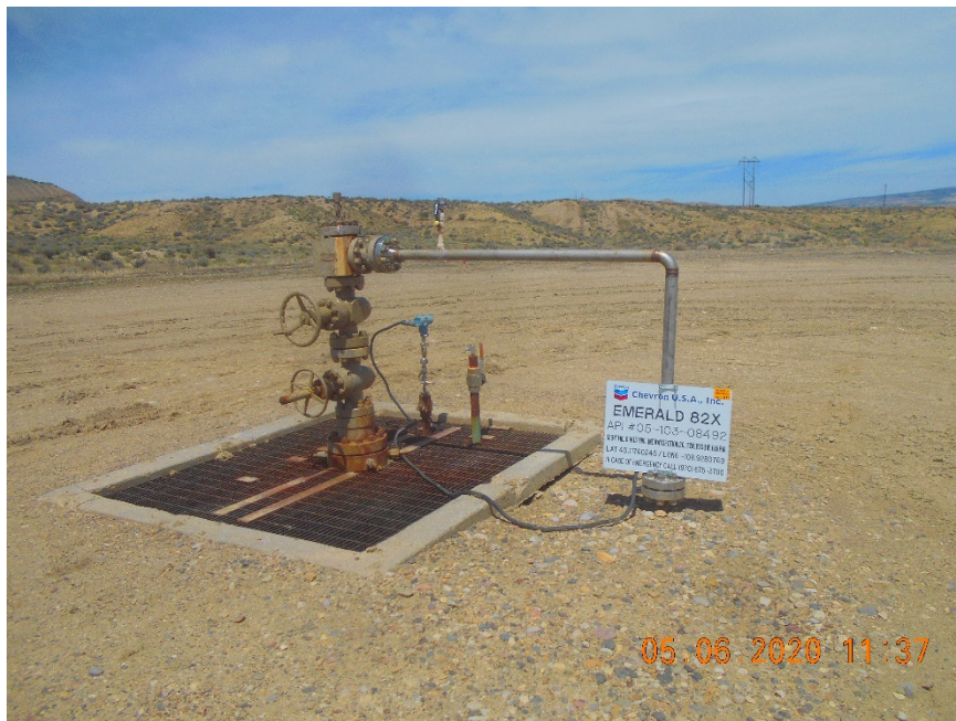
Injection wellhead
