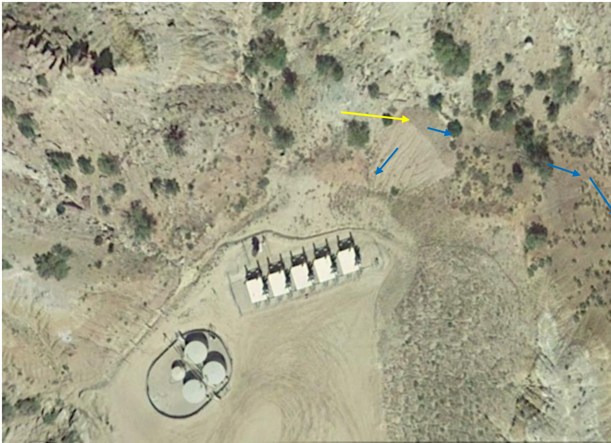
Photo 11: Google Earth aerial image. Photo shows areas where Operator appears to have pushed soils upon a hillside of the Location (yellow arrow). Insufficient BMPs, or BMPs missing from the slopes to prevent from erosion or sediment transport off Location. Blue arrows represent water flow direction.
