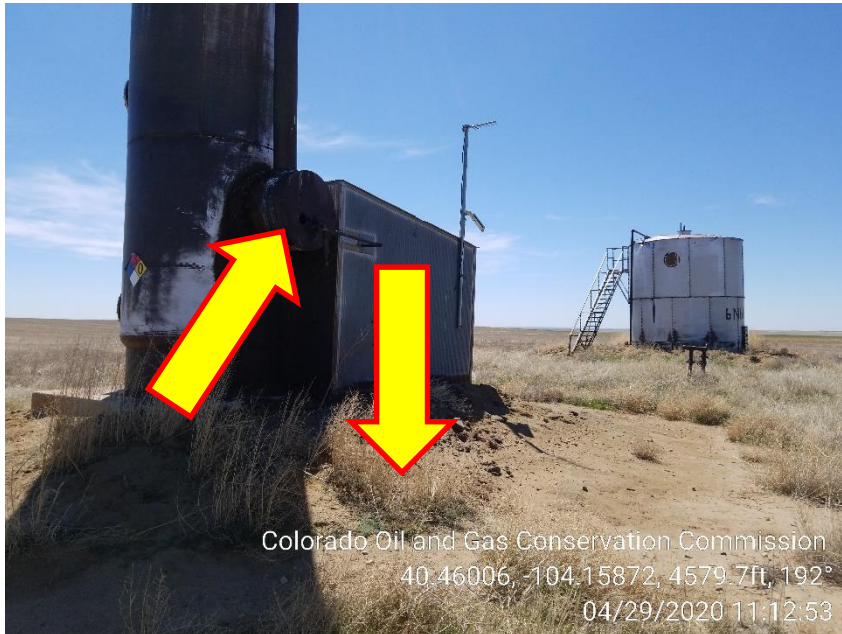
Photo 5 – Heater Treater, weeds, Wildlife screen missing
