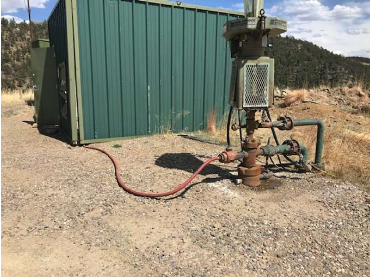
PHOTO 3: THE RED HOSE WAS RE-CONNECTED TO THE WELL HEAD AS THIS IS THE FUEL GAS LINE TO RUN THE PC ENGINE.
