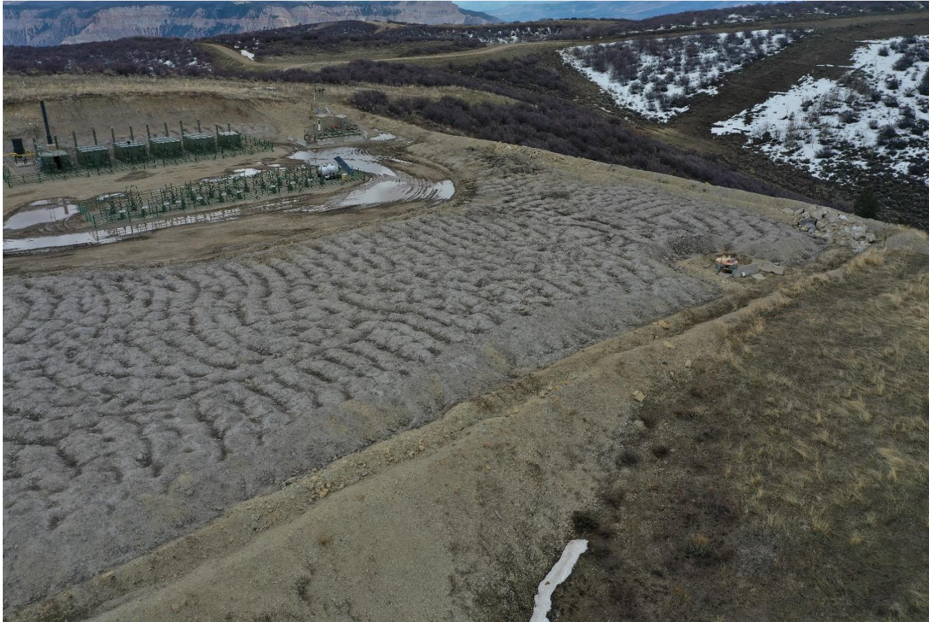
Photo 33: On 4/24/2020, Reclamation specialist Trujillo utilized a SUA to capture an aerial image of the Location; Photo taken from the south end of the Location, facing northeast. See comments under photo 29. Photo also show fill slopes on the south end of the location are predominantly exposed.
