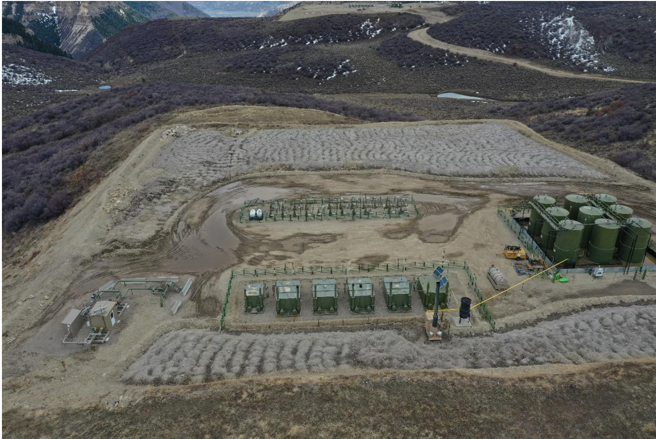
Photo 29: On 4/24/2020, Reclamation specialist Trujillo utilized a SUA to capture an aerial image of the Location; Photo taken from the north end of the Location, facing south. Photo shows large areas on the Northern and southern ends of the current pad where drill cuttings remain stored; these areas are not needed for production and are subject to 1003 interim reclamation. Photo also shows stormwater ponding on Location.
