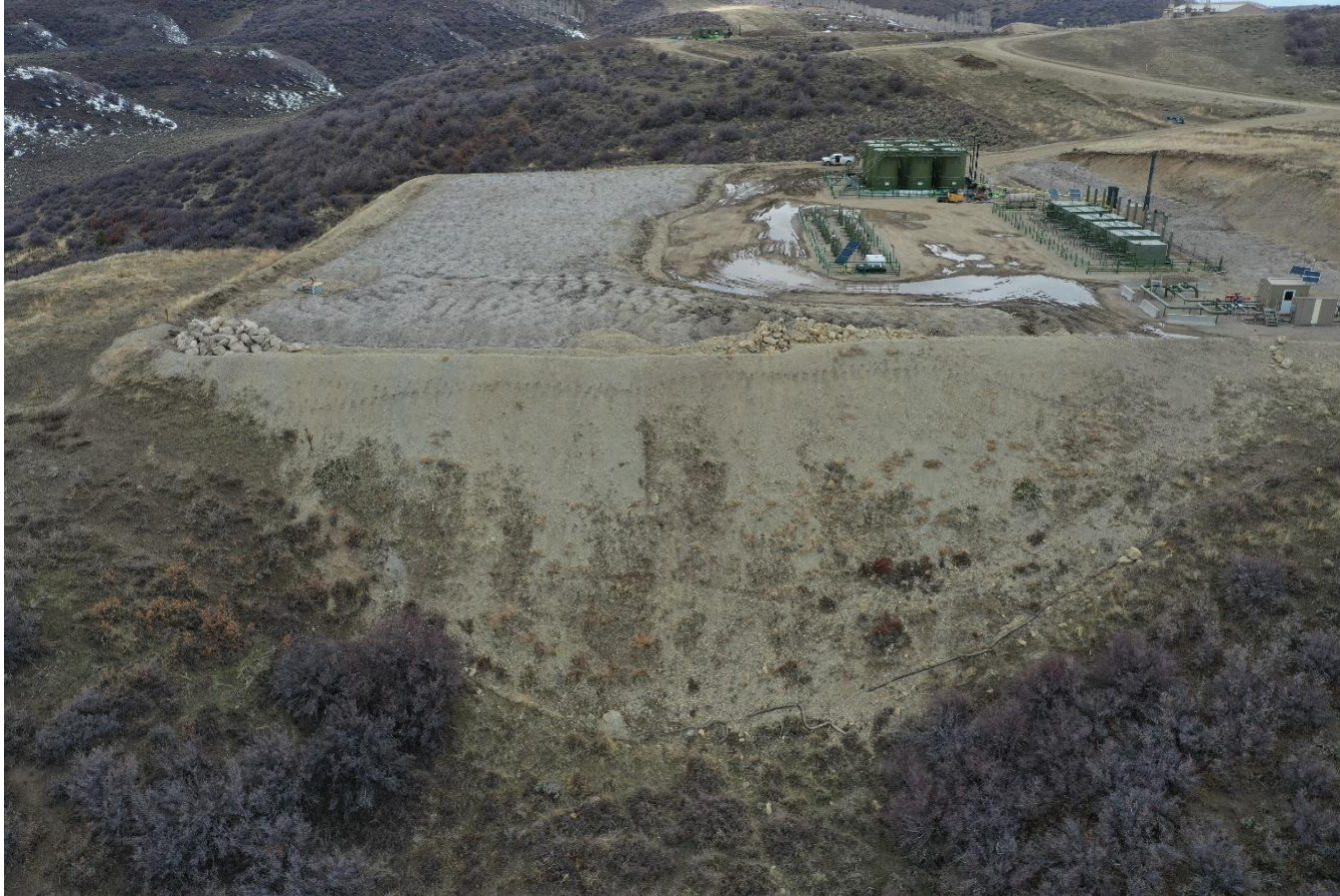
Photo 35: On 4/24/2020, Reclamation specialist Trujillo utilized a SUA to capture an aerial image of the Location; Photo taken from the east end of the Location, facing west. See comments under photo 29. Photo also show fill slopes on the east end of the location are predominantly exposed. Photo also show fill slopes on the west end of the location are predominantly exposed. Photo also shows perimeter BMPs are either in disrepair, or missing.
