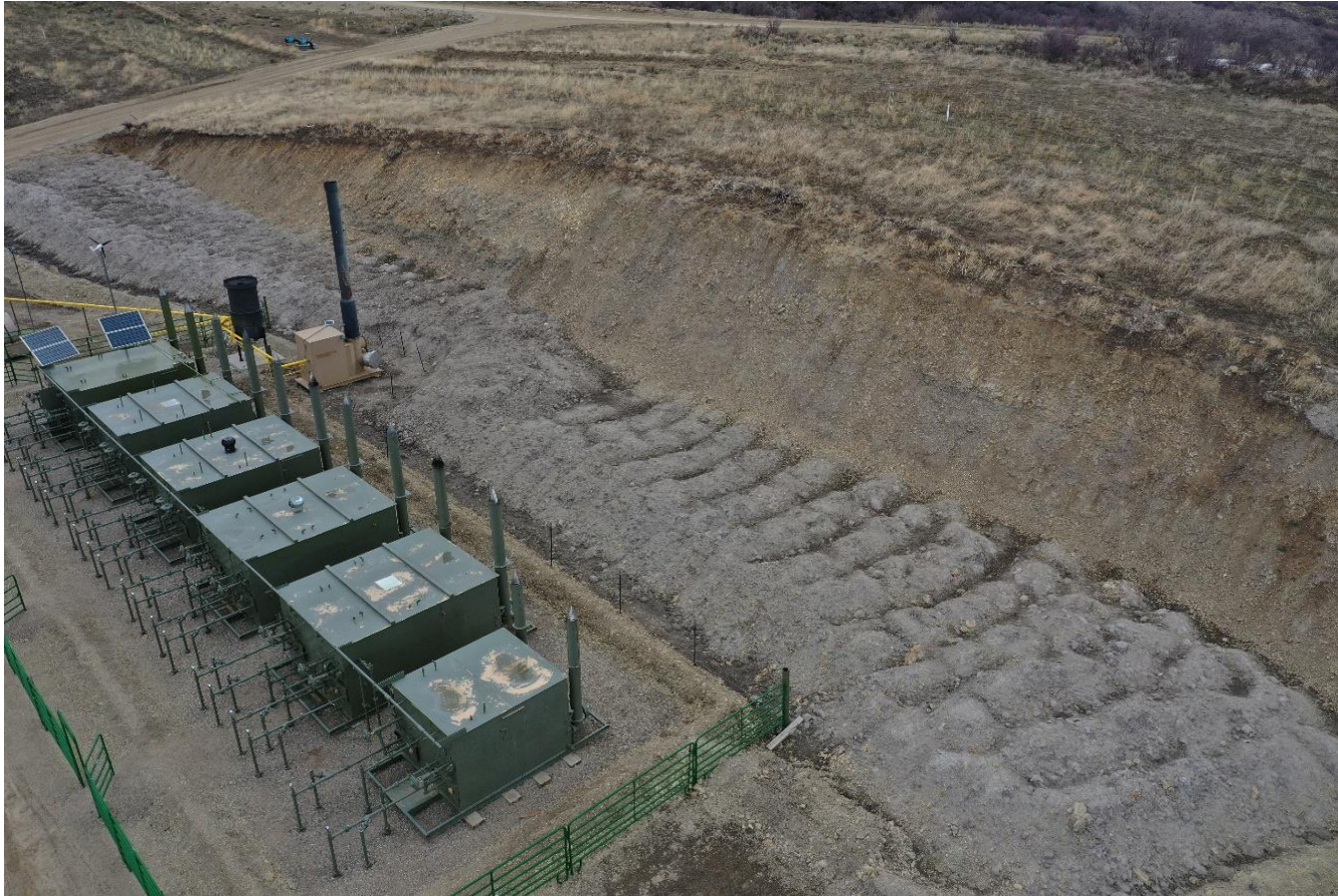
Photo 36: On 4/24/2020, Reclamation specialist Trujillo utilized a SUA to capture an aerial image of the Location; Photo taken from the north end of the Location, facing northwest. See comments under photo 29. Photo shows cut slope of the location is predominantly exposed.
