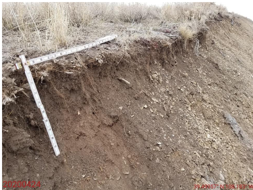
Photo 19: Photo shows the topsoil layer visible from the cut slope.
