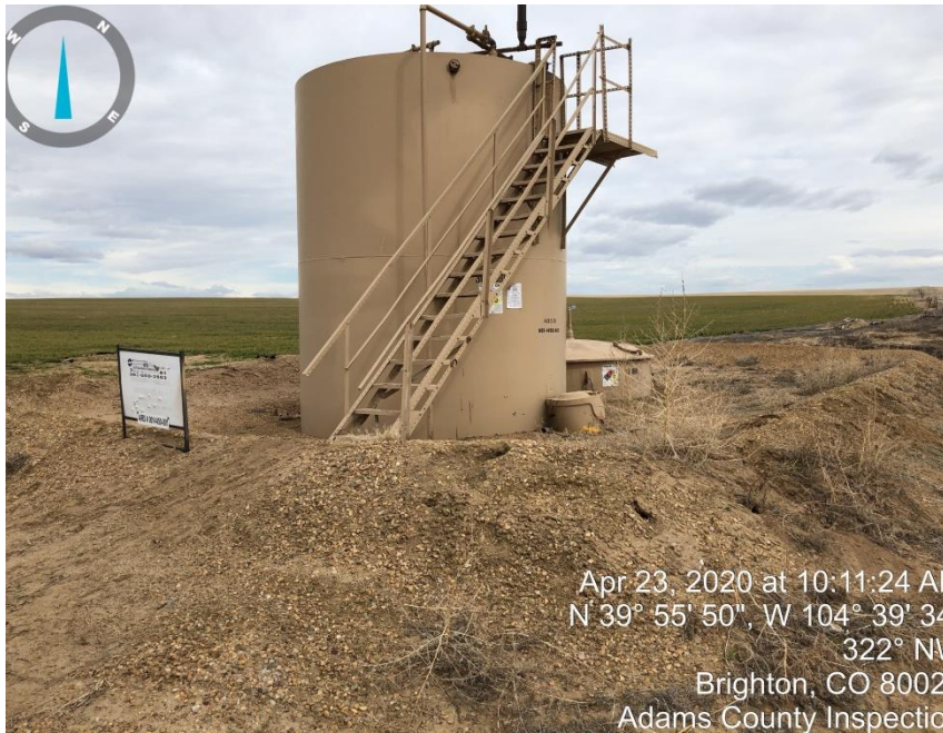
Photo#1 Production Tank and Produced water pit
