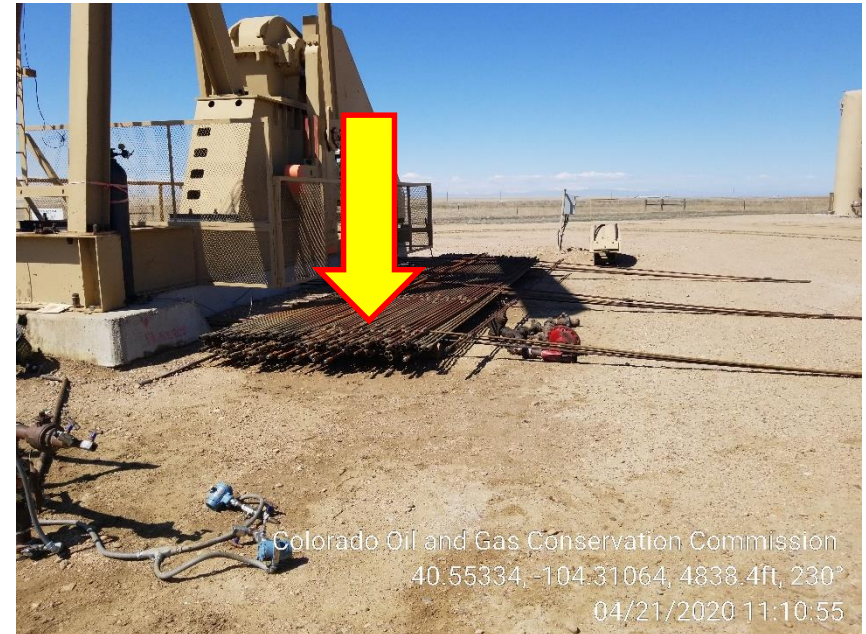
Photo 2 – Unused Rods at Pumping Unit
